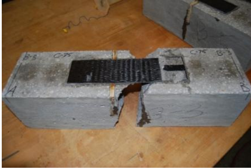
FIGURE 47. Typical Carbon Interfacial Shear Debond (Specimen B-3 a 75% Bond Area Specimen) with Same Fractured Concrete Material
