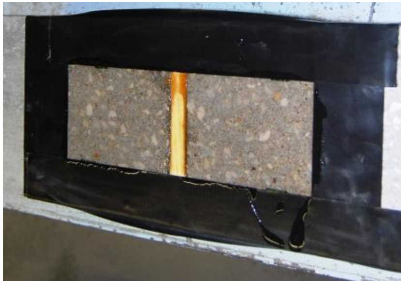
FIGURE 2B. Photo of ASTM-C78 Concrete Beam with 100% (Good) Bond Area.
