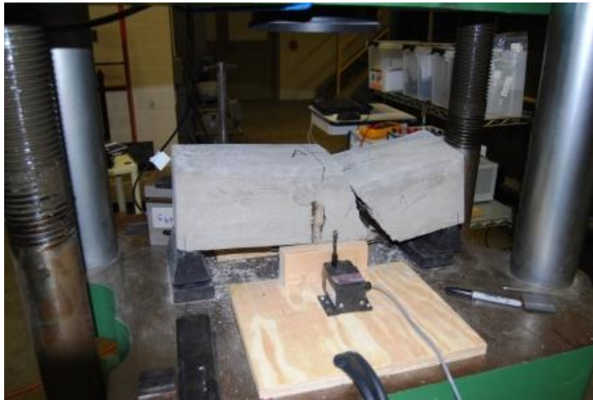
FIGURE 44. Typical Cracking Moment Type Failure at the End of FRP Reinforcement.
