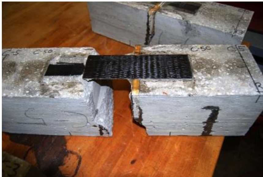
FIGURE 48. Typical Carbon Interfacial Shear Debond (Specimen C-5, a 50% Bond Area Specimen) with a Small Amount of Fractured Concrete Material
