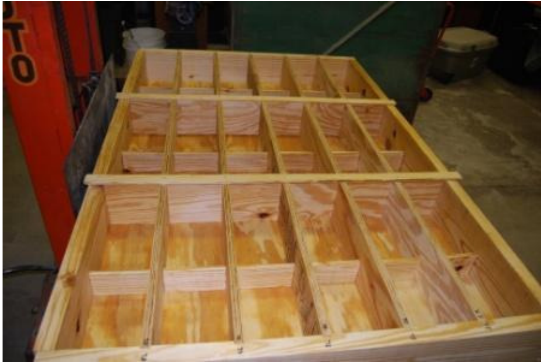
FIGURE 1. Wooden Forms Used to Construct Concrete Beam Test Specimens.
