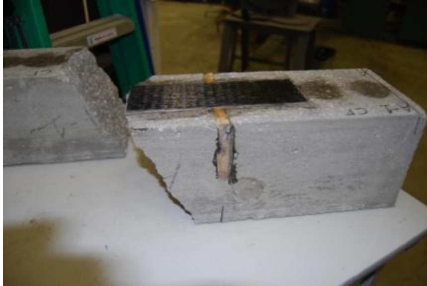
FIGURE 45. Typical Cracking Moment Type Failure at the end of the CFRP Reinforcement (Bottom Side).
