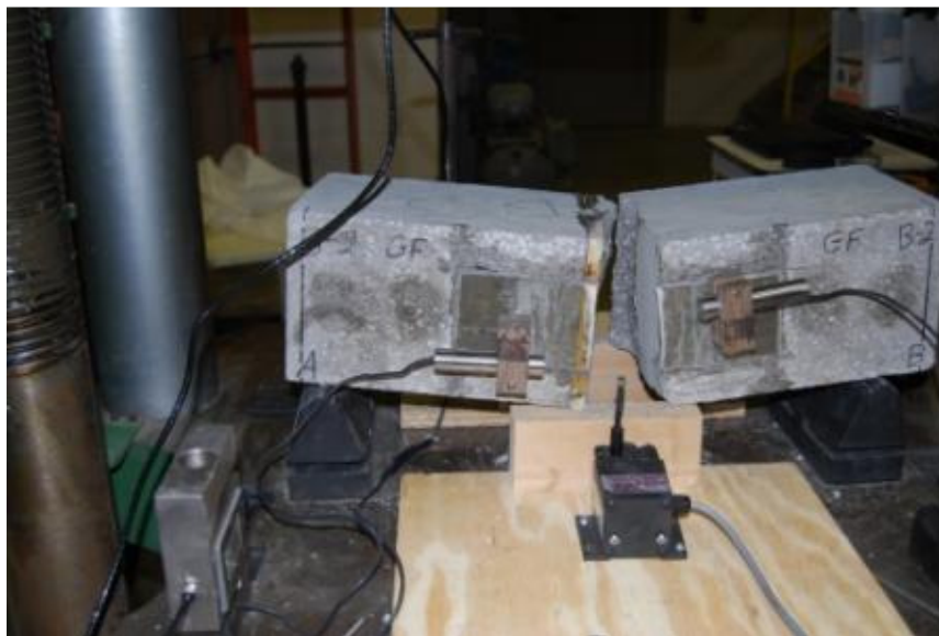
FIGURE 50. Typical Glass Fiber Rupture Failure
