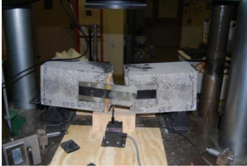
FIGURE 51. Typical Glass Interfacial Shear Debond Failure
